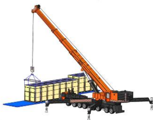
Long-side vertical package unloading with crane
