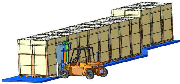
Long-side vertical package unloading with forklift
